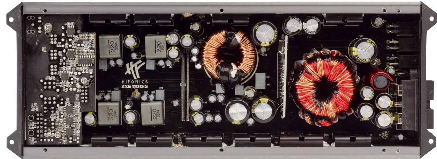
The ZXS1100/5 is much slimmer than the ZXR. On the left, you can see the encapsulated coils of the small channels, and in the middle, the giant coil for the bass channel
