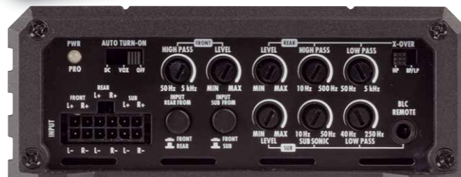
High-level or RCA harnesses dock to the Molex jacks
