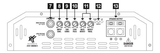
There are two RCA inputs on the **LINE INPUT**, each of which is controlled in mono. At the upper input **HIGH VOLTAGE** you can connect a high level signal from 1.0 to 9.0 volts, such as that provided by a DSP. The input **LOW VOLTAGE** is suitable for low level signals from 0.4 to 3.6 volts.
